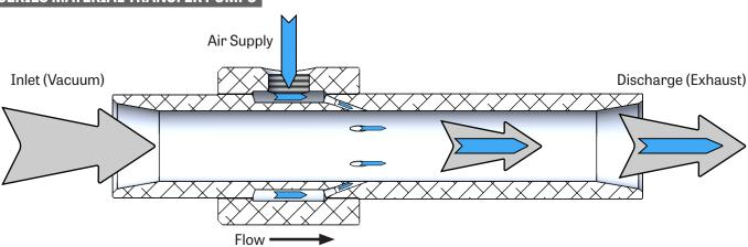
Direct Transfer Pumps use high velocity compressed air to generate a vacuum in the inlet of a smooth bore tubular body to drawn in bulk dry goods and then convey it in a turbulent air stream through a hose attached to the discharge end of the pump. Plastic pellets, powders, beans, peas, sawdust, and continuous fabric trimmings are only a few examples of the numerous items that can be transferred.
